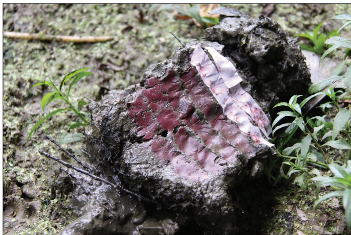
Figure 1. Example of \alpha,\alpha' -dipyridyl dye paper test strip. Note that the positive reaction is clearly visible both on the soil surface and on the paper test strip and that the reaction occurs across >60% of the soil layer. (Photo: USACE staff)
