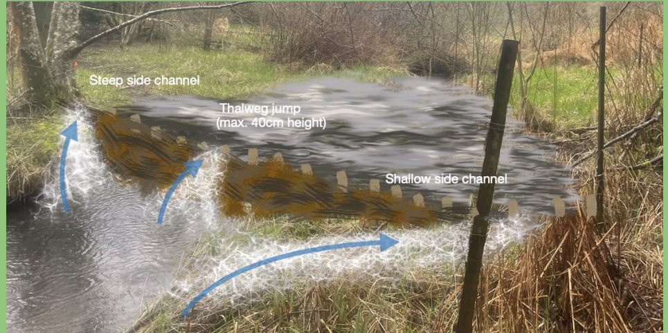
An imagined BDA at the southern extent of the Sapp Road study site with fish passage options based on Pollock et al (2022) (not including passage directly through the structure).
