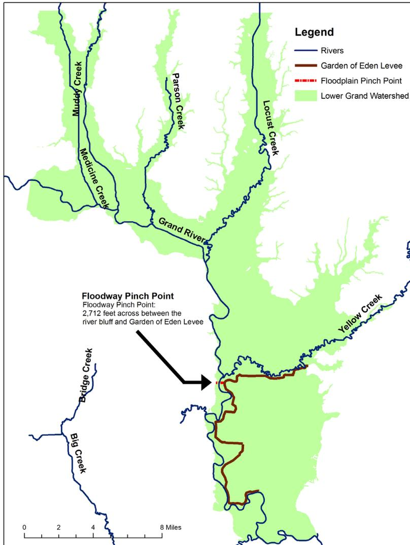
Figure 22. Constriction pinch point in the Grand River floodway caused by the Garden of Eden levee.
