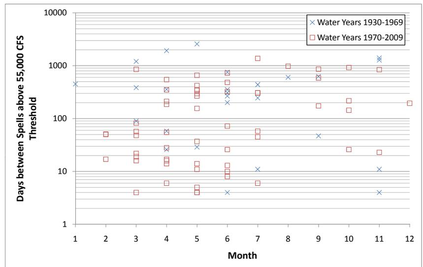
Figure 29. Occurrence of events with average daily discharge in the Grand River near Sumner, MO in excess of 55,000 cfs, shown by month for Water Years 1930-69 and 1970-2009 for USGS gauge #06902000.
